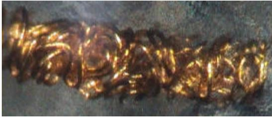
Figure 1: showing magnified view of a Fuzz Button.
