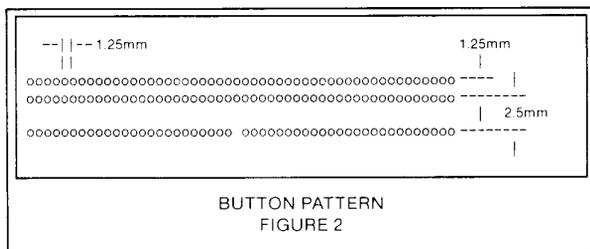
The buttons are inserted into 0.5mm holes in an .75mm epoxy glass carrier. The carrier has holes at each end to accept alignment pins. Epoxy glass was chosen as a carrier material to provide an expansion coefficient close to that of the multilayer board the connector will mate with. Contact pads on both the flexible cable and circuit board are .75mm diameter and plated with gold over nickel.
