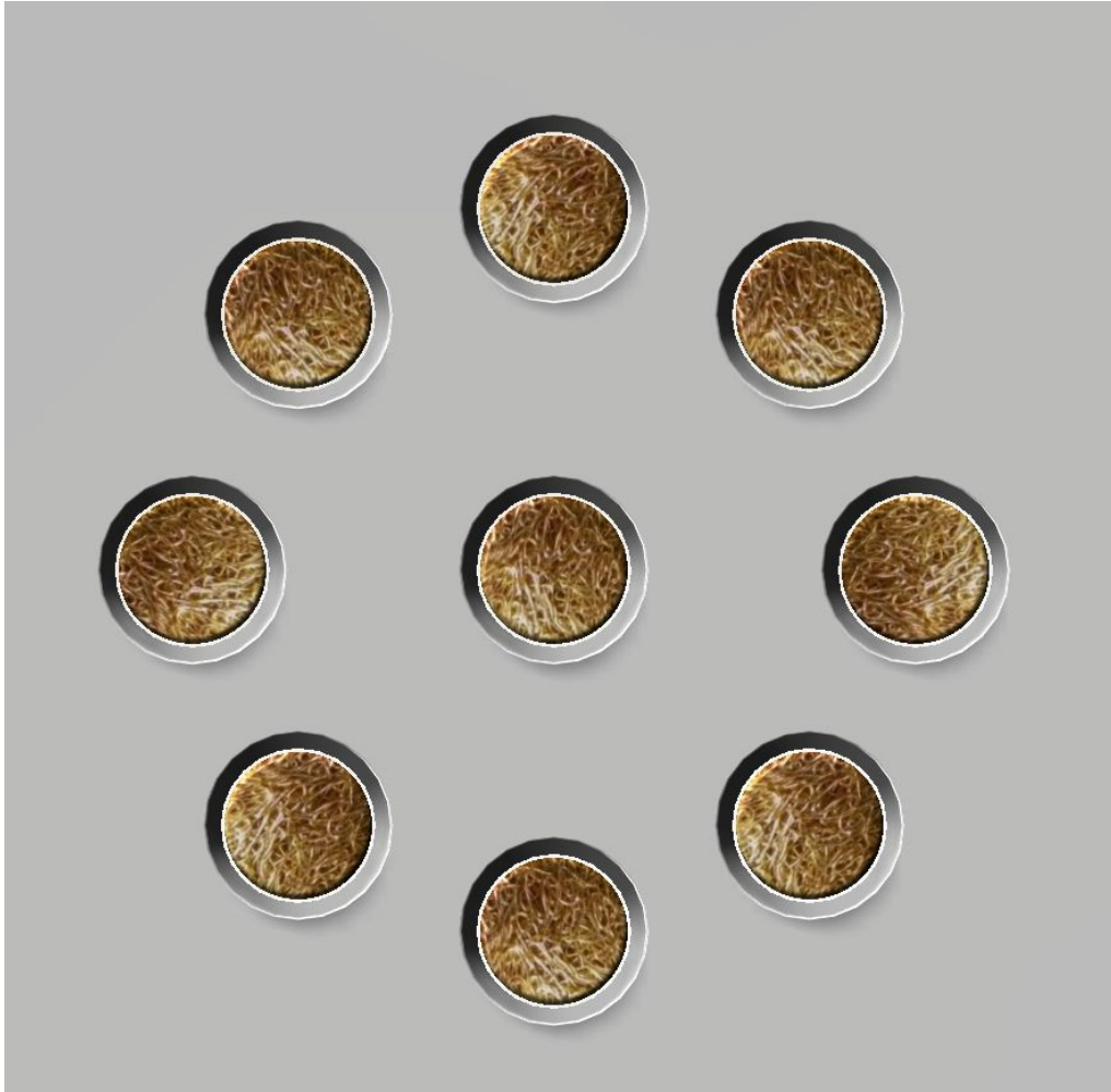
Figure 4 Ø0.020 Fuzz Button Interconnect Configuration
